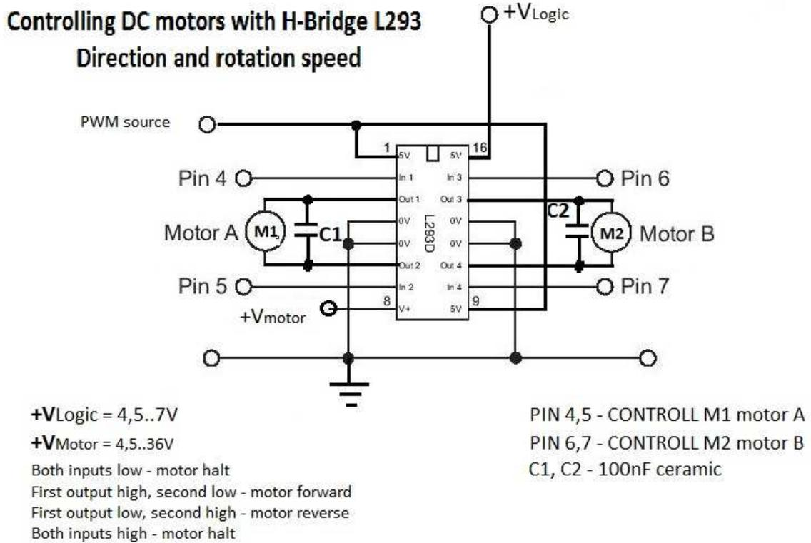
so now applying PWM source directly from the I/O pin from MCU we can control DC motor rotation speed.
