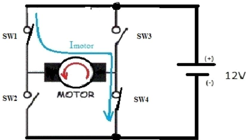
So as you can easily notice motor is spinning right when **switch 3** and **switch 2** is closed. And opposite in case of closing **switch 1** and **switch 4**. Need to be careful with simultaneous closing of **switch 1** and **switch 2**, the same **switch 3** and **switch 4** because short circuit will happen and definitely your battery will not like it at all.
