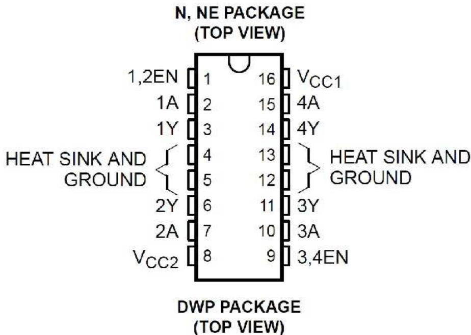
Every data that you will ever need you will find in its datasheet. I will present you only summary data that is needed for a simply current flow direction control. L293D allows control of any load with currents not bigger than 600mA; this current can rise up to 1A in case of using heat-sink.
