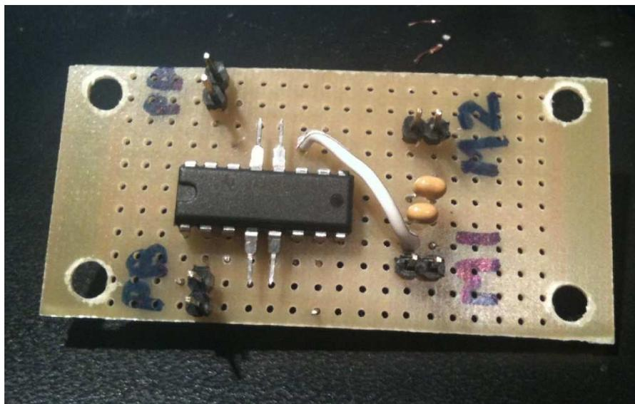
As you see I marked with PB and PD inputs for driver control and with M1 and M2 pins for motor's power.
