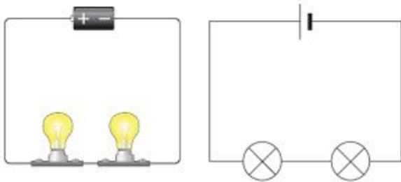
In a series arrangement of holiday lights, the bulbs are connected together in a daisy-chain, one after the other. Current flows through each bulb because it has no other paths to follow. Each bulb reduces the total current from the power source; so the more bulbs you have in a series circuit, the less current flows through the circuit.
