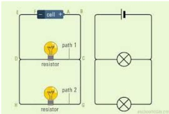
Light bulbs connected in a parallel circuit resemble the rungs of a ladder, in which each rung is connected to the ladder legs, and all rungs are parallel to one another. In this arrangement, current flowing through one bulb has no effect on the current in the others. Each additional bulb increases the total current, so a string with 20 bulbs uses 20 times the current of a single bulb.
