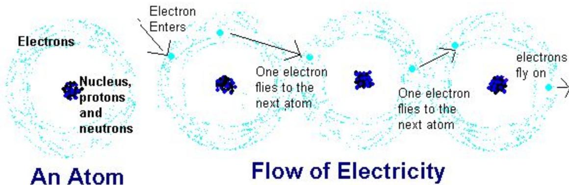
In an insulator, the atoms have few or no free electrons. The best example of an insulator is air. Electricity has a great deal of trouble traveling through air. This is evident if one were to cut a wire on a simple circuit leaving a gap between the two wires. Since air is an insulator, the electrons will not move across the gap.
